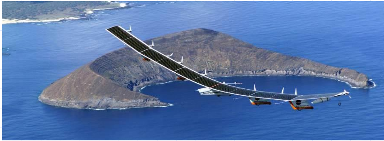
An experimental solar cell aircraft called Helios flying over the coast of Hawaii (Courtesy of NASA Dryden Research Centre)
