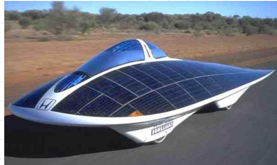
Honda's two seated Dream car is powered by photovoltaics. The Honda Dream was first to finish 3,010 km in four days in the 1996 World Solar Challenge. (Courtesy of Photovoltaics Special Research Centre, University of New South Wales, Sydney, Australia)
