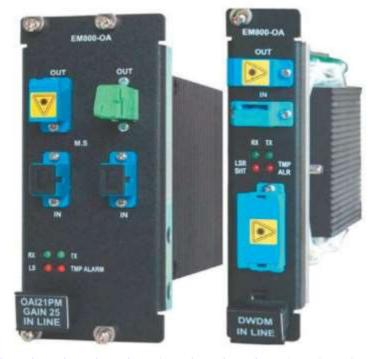
EDFAs (LambdaDriver®-Optical Amplifier Modules) with low noise figure and flat gain (to within ±1 dB) for use in DWDM over 1528 - 1563 nm. These amplifiers can be used for booster, in-line and preamplifier applications. (Courtesy of MRV Communications, Inc)
