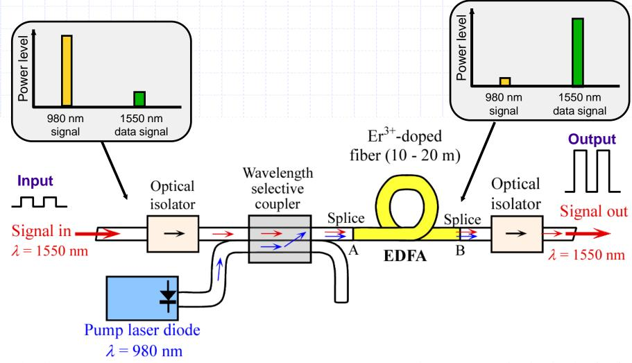
A simplified schematic illustration of an EDFA (optical amplifier). The erbiumion doped fiber is pumped by feeding the light from a laser pump diode, through a coupler, into the erbium ion doped fiber
