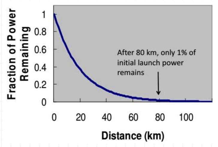
A light signal that is traveling along an optical fiber over a long distance suffers marked attenuation.
