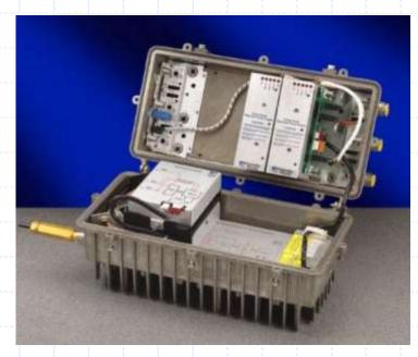
EDFA (Strand Mounted Optical Amplifier, Prisma 1550) for optical amplification at 1550 nm. This model can be used underground to extend the reach of networks; and operates over -40 °C to +65 °C. The output can be as high as 24 dBm (Courtesy of Cisco).
