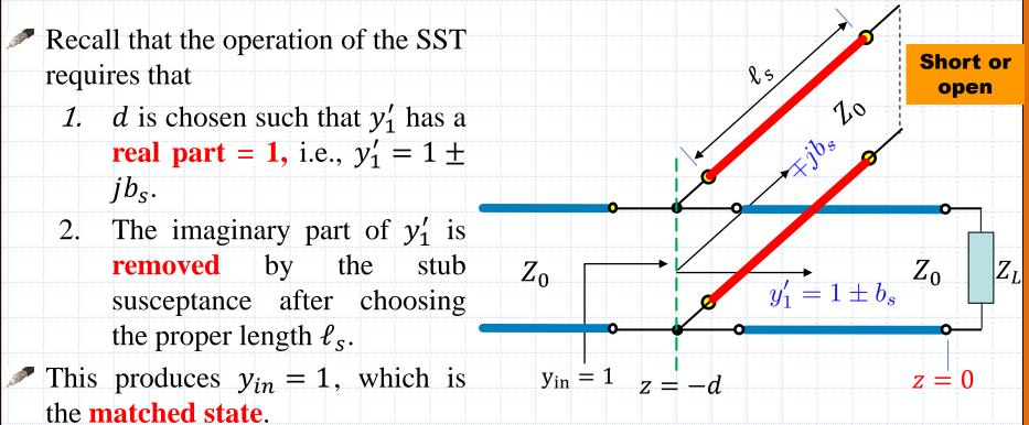
**Figure 5.2:** Using the Smith chart, design a shorted shunt, single-stub tuner to match the load  $Z_L = 60 - j80 \Omega$  to a T-Line with characteristic impedance  $Z_0 = 50 \Omega$ .
